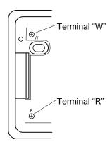
Figure 46 - Thermostat Base Terminal "W" and "R"
